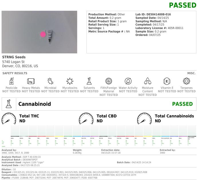
Full spectrum cannabinoid analysis utilizing High Performance Liquid Chromatography with DAD detection (HPLC-UV). Method SOP.T.90.010.CO for reporting. Lower limit of linearity for all cannabinoids is 1 mg/L.
